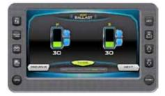
Set the ballast tanks by touching and sliding the finger up the tank area or by touching the [UP] and [DOWN] arrows alongside the tank area. Touch [NEXT] to continue.
