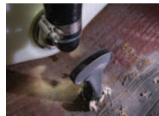
View beneath deck of properly installed center drain plug
