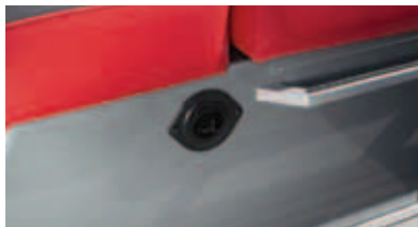
Starboard Cockpit Heater Vent
