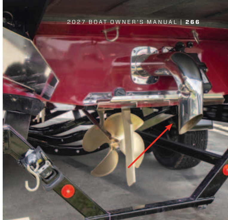
Underwater Exhaust Pipe
