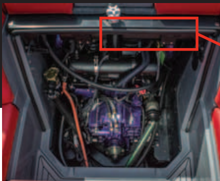
Supercharged 6.2L Ilmor Engine
