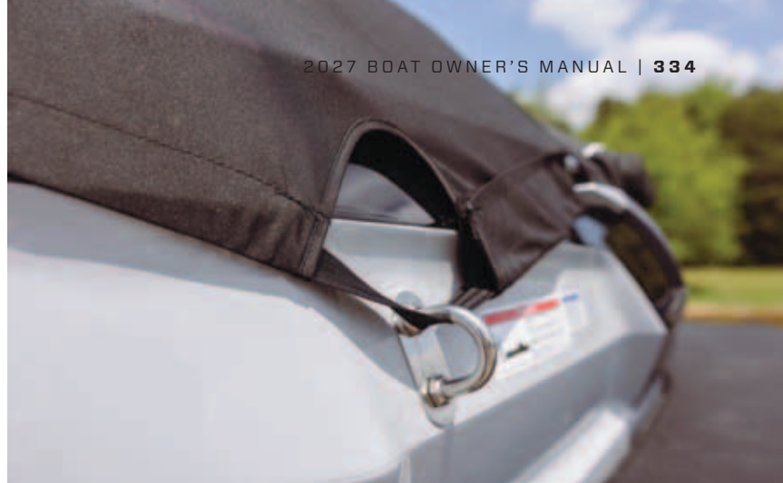
Pass-through Design, Buckles Through the Stern Eyes
