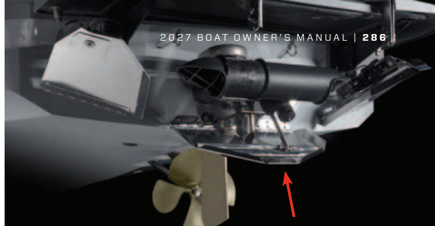
Attitude adjustment plate, also referred to as the center tab
