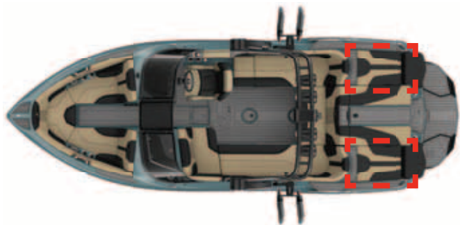
SurfStar Ballast Location on Equipped Models
