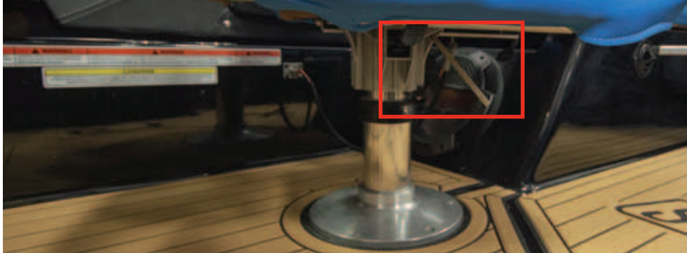
Gas Seat Assist Lever Under Helm Seat
