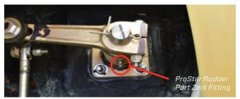
6. Using the flexible end of a grease gun, give two (2) full shots of white lithium grease to the zerk fitting on the steering tube pivot (circled above). Clean up any old grease purged from the areas.
