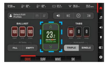
**Heading Out:** To prepare the boat for a riding session on the way to your favorite spot, navigate to Drive. The boat will default to 24 MPH and **AutoLaunch** Single will default to the ON position. Tap FILL ALL to start filling the ballast tanks.
