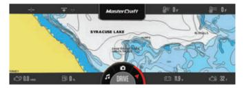
Located above the steering wheel on Dual Screen X and XT models, the PV1200 unit displays information relating to MPH, RPM, depth readings, temperature readings, battery charge, fuel levels, and oil status. It has 2 display options (Standard/ Wide) and 3 view modes (Media, Camera, and Navigation). These may be adjusted by selecting the toto on the PV1100 touchscreen.
