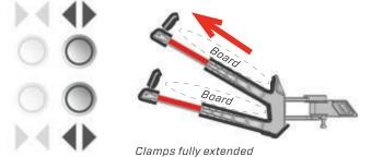
Pressing the inward facing arrows retracts the clamps back in. Top buttons will move the top rack clamps, the lower buttons will move the lower rack clamps.
