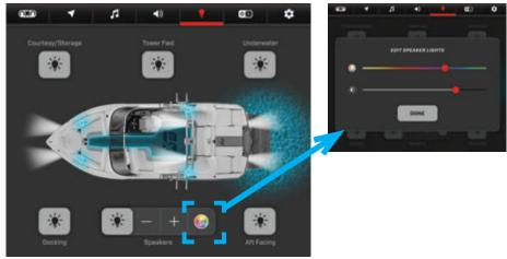
You may adjust the intensity of the speaker lights by touching the + and - buttons. Additionally, you may change the color of the lights by touching . After moving the slider to the desired color and intensity, touch **DONE**.
