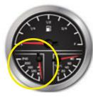
The temperature gauge indicates the water temperature inside the engine's cooling system as measured in degrees Fahrenheit. The normal operating temperature will range from 140 degrees Fahrenheit to 190 degrees Fahrenheit. Engines with electronic fuel injection also have a control circuit inside the engine control module that will cause the engine
