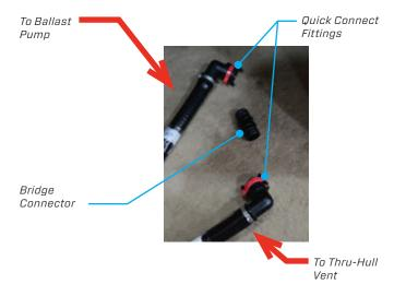
Some models have check valves equipped on the ballast lines. On such models pour a small amount of antifreeze into those vents (see guide to each boat in this Owner's Manual). The antifreeze will sit in the line during storage.
