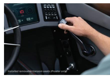
and umbrella. The engine will run with increased RPMs and can be increased or decreased by moving the lever. Returning the handle to the neutral position will bring the system back to neutral and reduce the engine RPMs to preset levels. This function should be done sparingly. Over-revving the engine for any extended period can cause undue wear and tear on the engine. Avoid advancing to wide-open-throttle and holding the RPMs at that level.
