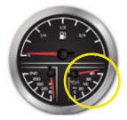
The engine oil pressure gauge indicates the pressure of the lubricating oil inside the engine. The average pressure ranges are between six (6) pounds per square inch (PSI) at 1000 RPM to 40 PSI or more at cruising-range speeds. A reading of pressure below 5 PSI at 1000 RPM may be caused by a low oil level or other potentially serious problems
