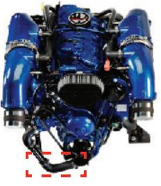
Image 3 Oil Cooler Location Under the Exhaust Manifold Image 3A Sea Strainer
