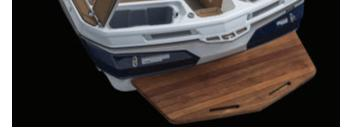
When oiling a platform, apply a coat of oil with a wet cloth, work into the seams, end grain and edges. Allow the oil to set approximately 15 minutes and then wipe off the excess oil with a dry cloth. Do not let the oil dry on the platform in the sun. Excess oil should be removed with a dry cloth.
