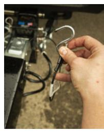
up on the push rod release bracket located on the underside and behind the hitch ball socket. This allows the bead to retract into the actuator. This releases the trailer brakes. Install a new clip on the breakaway cable in front of the bead.
