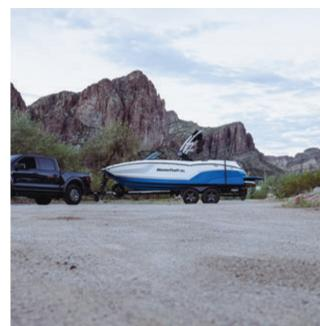
Do not tow the boat with wakeboards, skis or other gear left on the board tower racks. Doing so may void the warranty and cause damage to the boat or to vehicles following behind as boards and/or racks may become disengaged.
