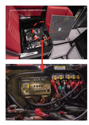
To reset PDM circuits, access the "Diagnostics" menu on the dash screen. Find the toggle for the circuit and reset it. (If the circuit has tripped, the menu will display an orange, red, or yellow icon beside the problematic circuit, depending on the issue encountered.) Allow a few seconds to pass while the digital switching resets. Turn the circuit back on. If the circuit continues to trip, there is a problem requiring urgent attention from an authorized dealer.
