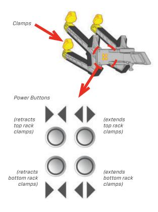
Pressing the outward facing arrows extends the clamps. Top buttons will move the top rack clamps, the lower buttons will move the lower rack clamps.
