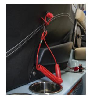
On April 1, 2021 a new federal law went into effect that requires the operator of a boat, less than 26 feet in length, with an installed Engine Cut-Off Switch (ECOS) to use the ECOS link. The link is usually a coiled bungee cord lanyard clipped onto the operator's person, Personal Flotation Device (PFD) or clothing and the other end attached to the cut-off switch. The law applies on all "Navigable Waters of the US".
