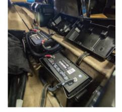
water-and-baking-soda solution that is used to clean the terminals. Rinse with fresh water and dry with a cloth.
