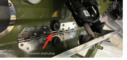
All boats (except ProStar) have two drain plugs, which allow water to be drained from the boat when the boat is OUT of the water. There is a center T-handle drain (the only one for a Prostar) and a transom drain plug. When out of the water, on a trailer or lift, water can normally be drained into the bilge system by opening the center drain.
