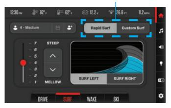
Any adjustments made to your surf wave will appear on the graphic to the right of the adjustment controls. Whenever new adjustments are made, a readiness timer will indicate the load time.
