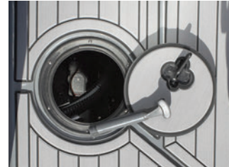
Open deck hatch at helm to access drain plug
