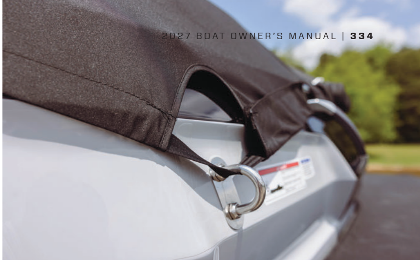
Pass-through Design, Buckles Through the Stern Eyes
