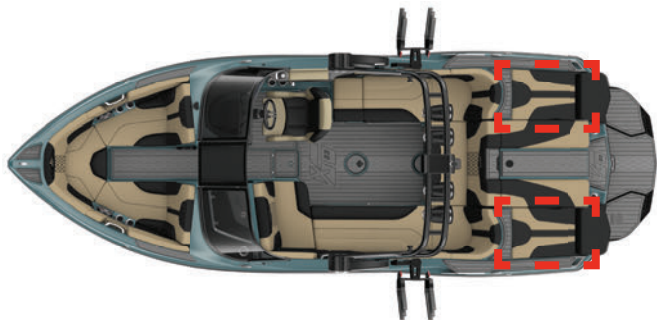
SurfStar Ballast Location on Equipped Models
