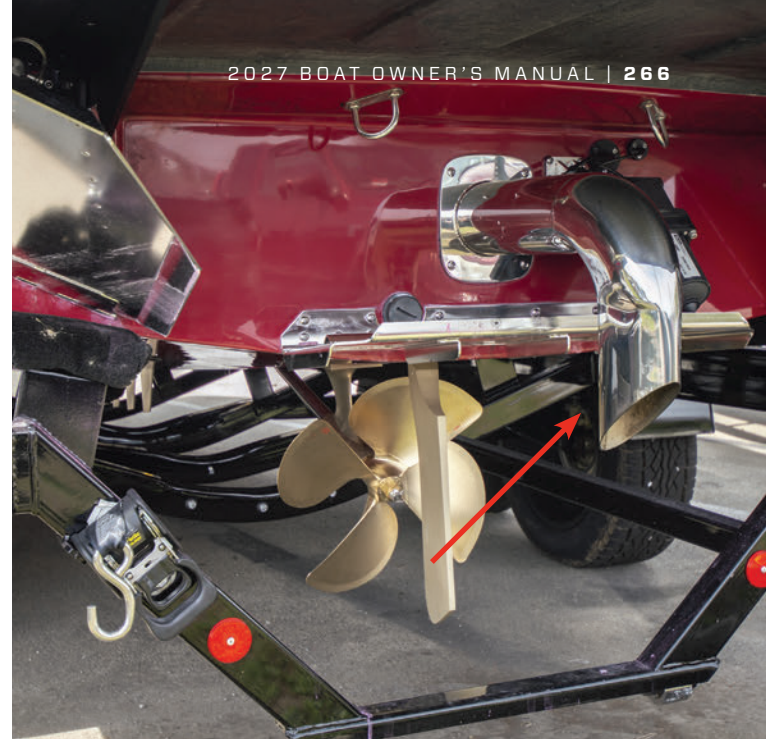
Underwater Exhaust Pipe
