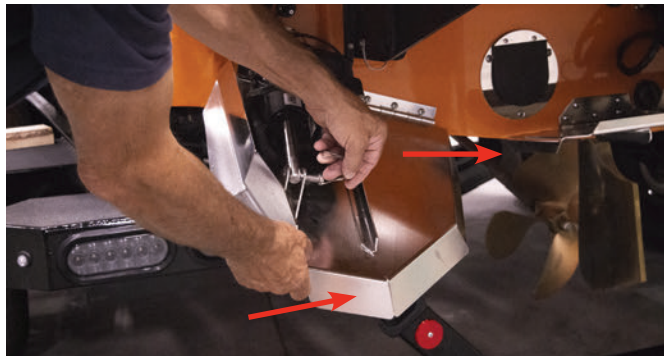
3A. Lift tab and pull pin barrel
