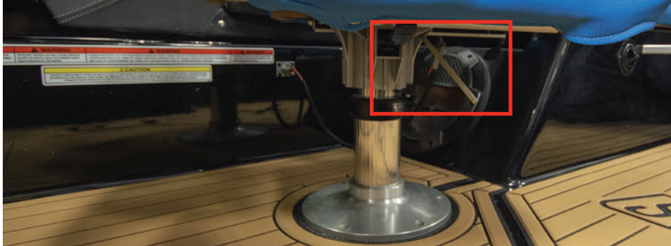
Gas Seat Assist Lever Under Helm Seat
