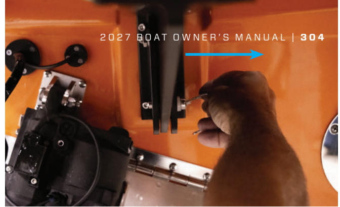
4B. Remove platform bracket pins
