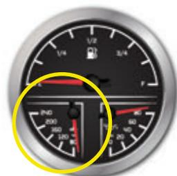
The temperature gauge indicates the water temperature inside the engine's cooling system as measured in degrees Fahrenheit. The normal operating temperature will range from 140 degrees Fahrenheit to 190 degrees Fahrenheit. Engines with electronic fuel injection also have a control circuit inside the engine control module that will cause the engine
