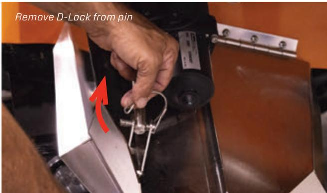
*Lift tab and pull pin barrel*
