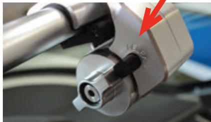
To lock in place, turn the lock knob to the marked lock position, the release button will pop out. To unlock, push the black release button and the lock knob will spring open. Raise or lower the mirror, and re-lock it in place.
