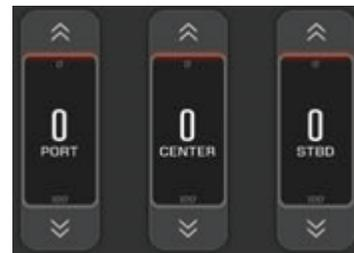
Make adjustments to each tab by touching the up and down arrows or sliding your finger up or down the slider bar.
