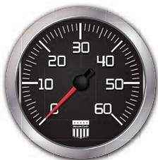
The speedometer indicates the forward speed of the boat in miles per hour (unless the boat is equipped with a speedometer that measures kilometers per hour, which is available in the optional European package.)
