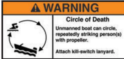
*On April 1, 2021 a new federal law went into effect that requires the operator of a boat, less than 26 feet in length, with an installed Engine Cut-Off Switch (ECOS) to use the ECOS link. The link is usually a coiled bungee cord lanyard clipped onto the operator's person, Personal Flotation Device (PFD) or clothing and the other end attached to the cut-off switch. The law applies on all "Navigable Waters of the US."*
