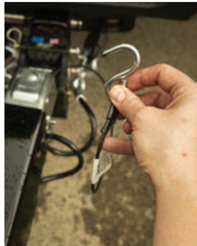
up on the push rod release bracket located on the underside and behind the hitch ball socket. This allows the bead to retract into the actuator. This releases the trailer brakes. Install a new clip on the breakaway cable in front of the bead.
