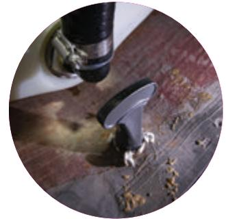
*View beneath deck of properly installed center drain plug*
