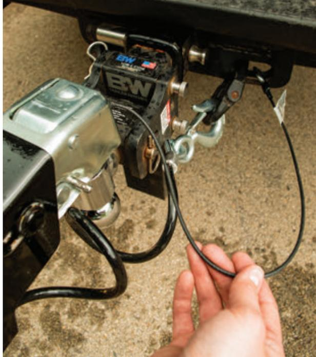
**How to install the breakaway cable clip:** The breakaway cable clip is installed on the breakaway cable to prevent inadvertent pressurization of the trailer brakes if the cable is lightly pulled by accident. If the breakaway cable is pulled during an emergency situation, the clip will be destroyed. The breakaway system must be reset by pushing up on the tab located under the coupler and the clip must be replaced. Contact your Authorized MasterCraft dealer for a replacement clip.
