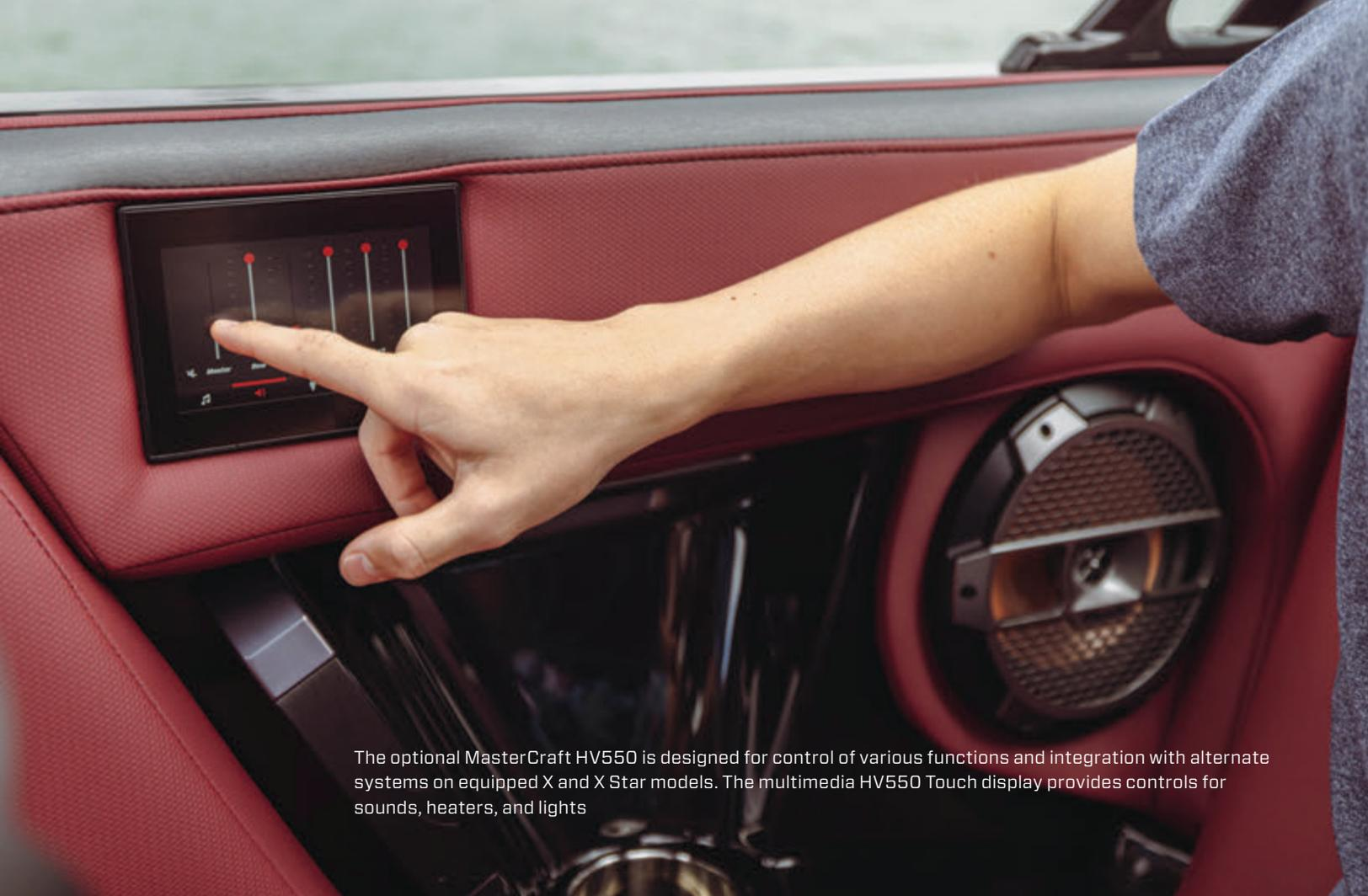
The optional MasterCraft HV550 is designed for control of various functions and integration with alternate systems on equipped X and X Star models. The multimedia HV550 Touch display provides controls for sounds, heaters, and lights
