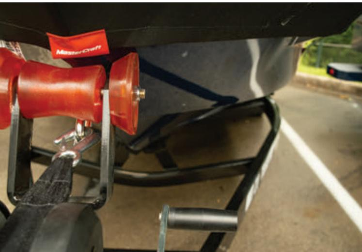
Using a damaged or worn winch strap may result in serious injury or damage. Check the winch straps frequently. The strength in these can deteriorate from exposure to weather, ozone and ultraviolet light (direct sunlight). If a strap becomes frayed or worn, replace it immediately with a new one.
