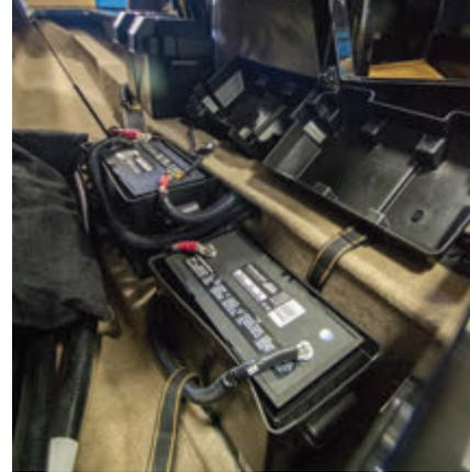
water-and-baking-soda solution that is used to clean the terminals. Rinse with fresh water and dry with a cloth.
