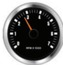
The tachometer indicates the engine speed in crankshaft revolutions per minute (RPM). See the Engine section of this Owner's Manual for important information regarding proper operating RPM levels, particularly during a boat break-in period.
