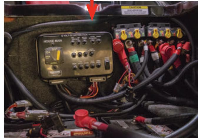
To reset PDM circuits, access the “Diagnostics” menu on the dash screen. Find the toggle for the circuit and reset it. (If the circuit has tripped, the menu will display an orange, red, or yellow icon beside the problematic circuit, depending on the issue encountered.) Allow a few seconds to pass while the digital switching resets. Turn the circuit back on. If the circuit continues to trip, there is a problem requiring urgent attention from an authorized dealer.
