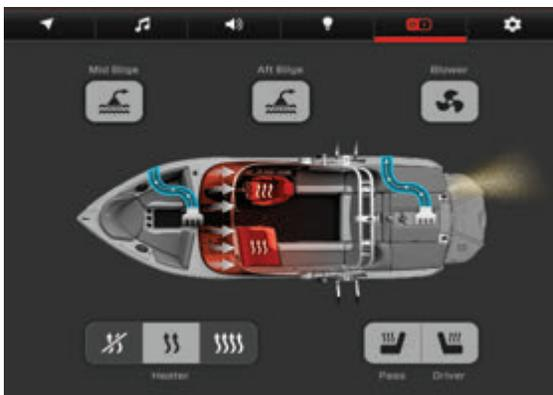
*Please note: When the ignition key is turned to the “on” position, the blower will automatically activate and run for exactly four (4) minutes. If you would like to turn the blower on manually, you may do so from the Accessory Switches Page.*
