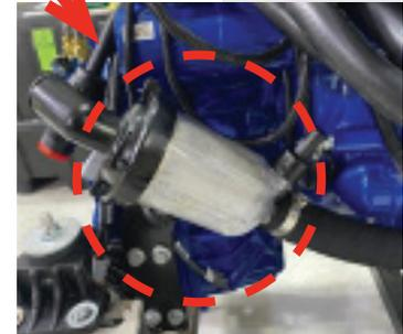
4. Remove the anode from the back of the cooler and drain the raw water. (Reference images 2 and 2B.)
