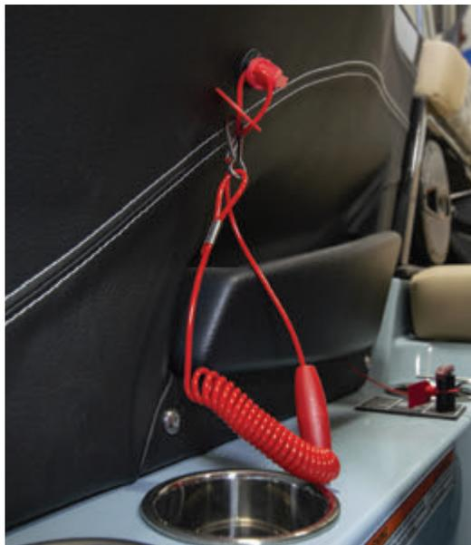
*On April 1, 2021 a new federal law went into effect that requires the operator of a boat, less than 26 feet in length, with an installed Engine Cut-Off Switch (ECOS) to use the ECOS link. The link is usually a coiled bungee cord lanyard clipped onto the operator's person, Personal Flotation Device (PFD) or clothing and the other end attached to the cut-off switch. The law applies on all "Navigable Waters of the US".*
