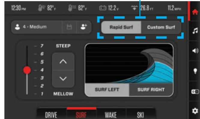
Any adjustments made to your surf wave will appear on the graphic to the right of the adjustment controls. Whenever new adjustments are made, a readiness timer will indicate the load time.
