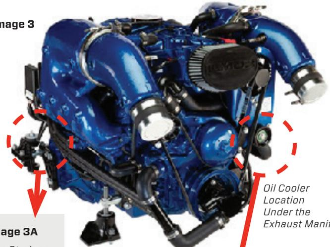
*Oil Cooler Location Under the Exhaust Manifold*
