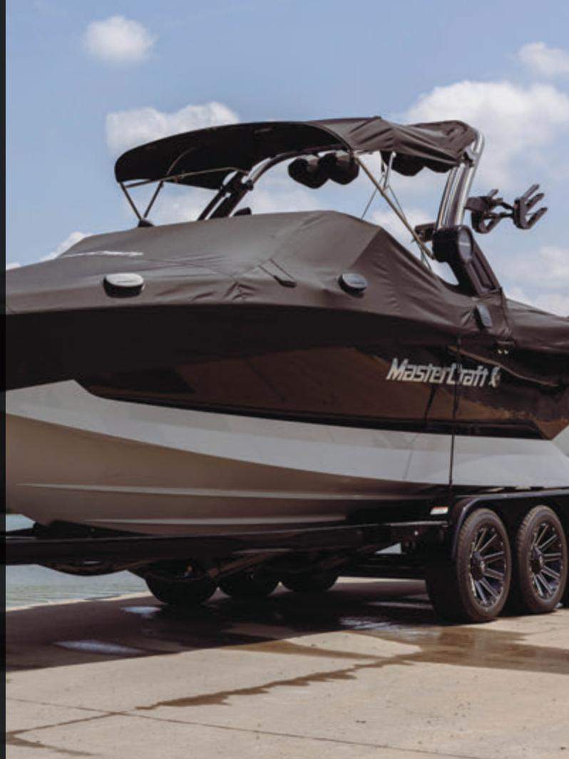
Note that towing with unapproved covers on the boat may result in damage to the gel coat. MasterCraft recommends using only approved towable mooring covers when towing. Other canvas covers are available only through authorized MasterCraft dealers for a variety of uses.
