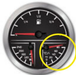
The engine oil pressure gauge indicates the pressure of the lubricating oil inside the engine. The average pressure ranges are between six (6) pounds per square inch (PSI) at 1000 RPM to 40 PSI or more at cruising-range speeds. A reading of pressure below 5 PSI at 1000 RPM may be caused by a low oil level or other potentially serious problems
