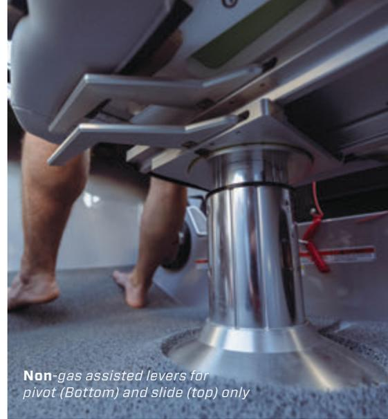
*Non-gas assisted levers for pivot (Bottom) and slide (top) only*
