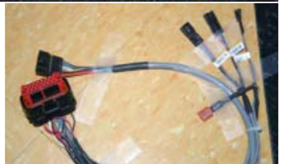
*Step 19:* Connect the throttle wire from the engine connector to the display side connector.
