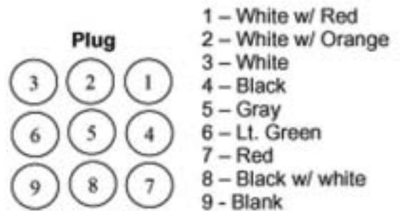
**Step 16:** Replace the engine-side 9-pin connector from the Perfect Pass master module with the provided engine connector harness.
