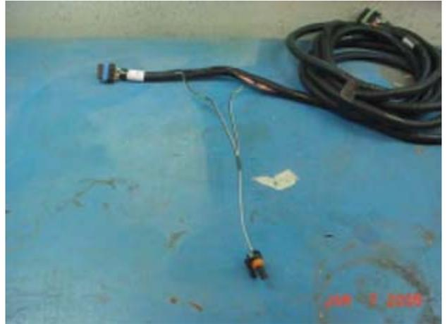
Step 10: Heat the shrinkable connectors to ensure a good seal between the connections.
