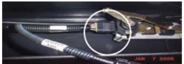
Step 12: Connect the jumper harness into the shift position wire harness.
