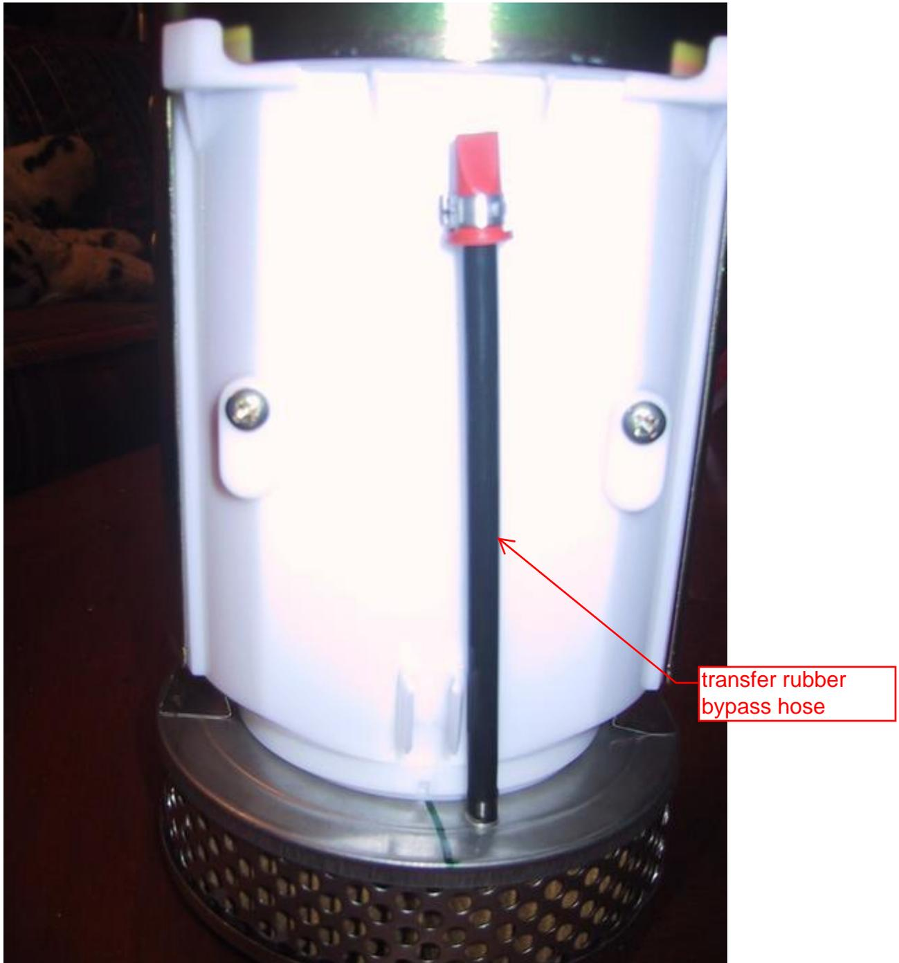
Transfer rubber flange from old pump suction to new
