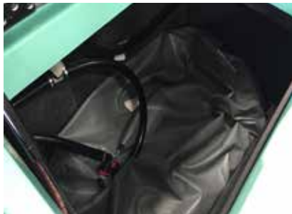
Additional sundeck compartment ballast bag
